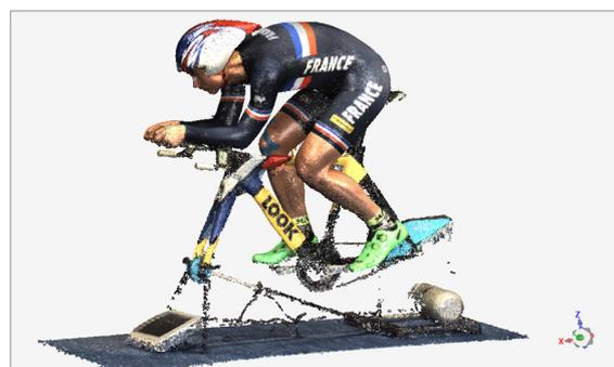
Figure 2: Model obtained with the Faro freestyle 3D.
